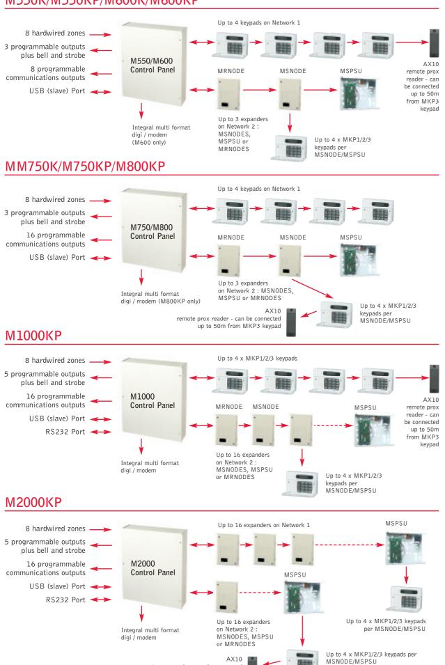
remote prox reader - can be connected up to 50m from MKP3 keypad 田
